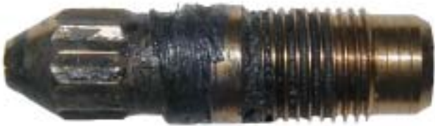
Hot runner nozzle encrusted with residue build-up
