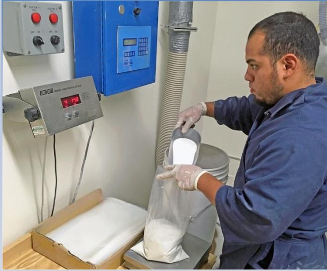
Micro-abrasives easily attract moisture due to their high ratio of surface area to volume. As water molecules stick to a particle's surface, a natural bond forms. This bond causes abrasive particles to clump. Clumps interrupt the flow of an abrasive stream, or worse, clog a blaster.
