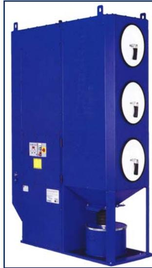
These centralized dust collection systems are designed for heavier requirements such as use of multiple blasters, continuous use of a DirectFlo or PowerFlo® or with automated systems. They are equipped with a sensor that triggers the automatic cleaning as needed, while in operation. The filter design and automatic cleaning increase the efficiency of the filters, which means longer life.
