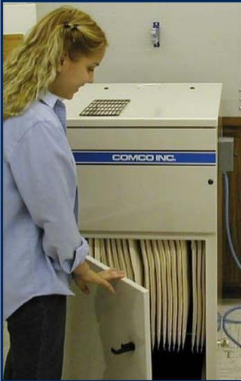
Cloth style dust collectors are freestanding units that do not require special installation. Their compact design includes everything necessary for connection to the back of the workstation. Models are available for systems using a single MicroBlaster® intermittently up to the larger DirectFlo or PowerFlo® production model blasters.
