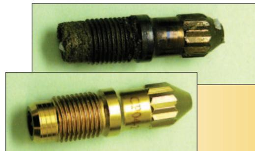
**Figure 4.** A closeup of pump nozzle tips before and after cleaning with the microblasting technique.
