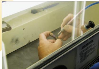
After a mold has been machined into a steel cavity with EDM or another method, it requires a final finish. A technology known as microblasting is used to create some of these finishes. Certain plastics release more easily from a frosty finish and some require a slick finish. Microblasting can texture small, deep cavities that larger bead blasters can't reach, but it also finds application in cleaning
