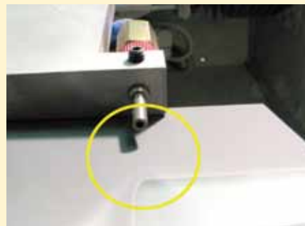
Figure 2. Testing nozzles, angles, pressures and distance between the solar cell and the blast can be done manually and the data used to create fixturing for the automated system.
