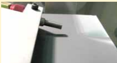
Figure 1. The unique properties of high-energy abrasive particles make microblasting ideal for CIGS solar cell applications. It cuts without heat or vibration and can selectively remove layers without damaging underlying layers or surfaces.
