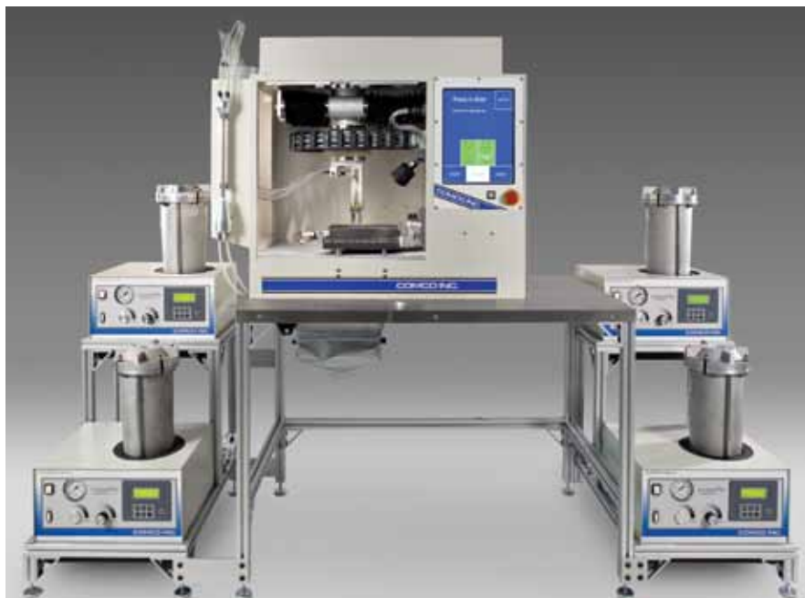
Figure 6. A wide range of microblasting formats are available for integration into customized automation production lines, depending on the end result desired.
