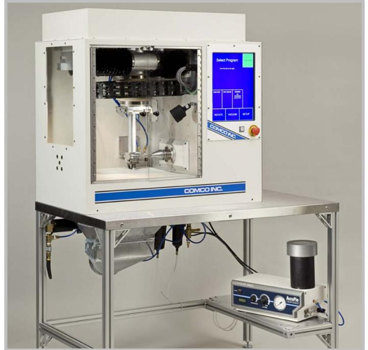
along the axis of a stent can be rounded with micro-abrasive blasting to eliminate the sharpness of the strut's edge.
