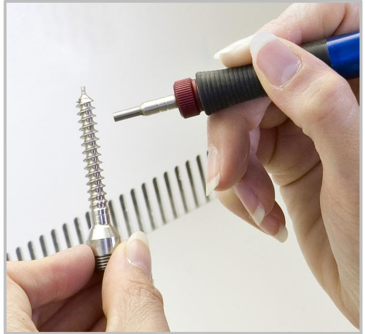
Micro-abrasive blasting is also used to finish the screw head. Whether hex- or square-fit, the screw broach may have small burrs that could break off when the screw is implanted.
