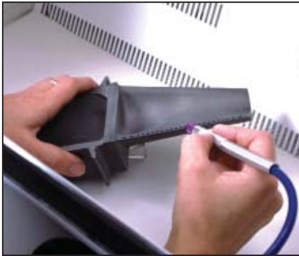
Whether a manual (shown) or multiple-fixtured semi-automated system, the process is basically the same. Comco MicroBlasting mixes an abrasive media in granular form with a jet of clean, dry air that is propelled through a pencil-like stylus tipped with a small nozzle.
