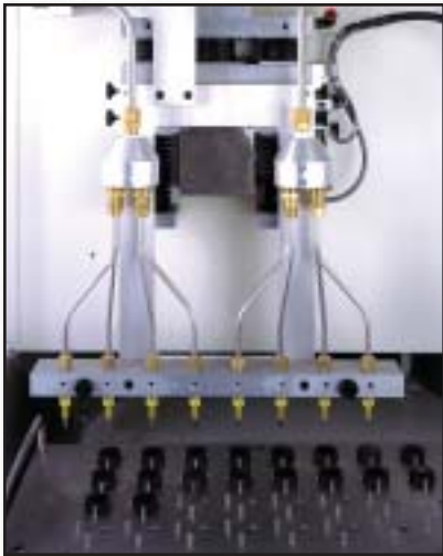
New high-power Comco MicroBlasters are capable of running nozzle array configurations for semi-automated applications. Fixturing shown is designed to present product to the nozzles.
